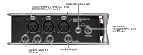
**INPUTS 1-3 FEMALE XLR JACKS** Active-balanced analog microphone or line-level inputs. Input 1 can also accept AES3 or AES42 signal. [pin-1 = ground, pin-2 = hot (+), and pin-3 = cold (-)].
