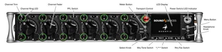
**CHANNEL TRIM** Turns the channel on/off and sets the input sensitivity for the channel. To conserve power, turn off unused channels by rotating channel trim fully counterclockwise.
