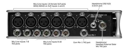
**INPUTS 1-6 FEMALE XLR JACKS** Active-balanced analog microphone or line-level inputs. Inputs 1 and 6 can also accept AES3 or AES42 signal. [pin-1 = ground, pin-2 = hot (+), and pin-3 = cold (-)]
