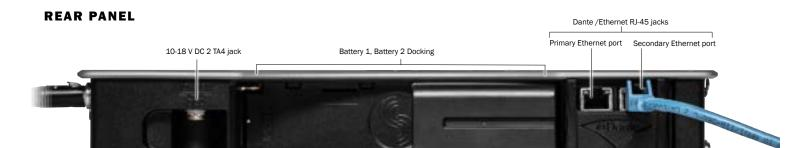
**10-18V DC2 TA4 JACK** Accepts DC voltages from 10–18 V for powering. [pin-1- GND, pin-2- Smart Battery DATA, pin-3- Smart Battery CLOCK, pin-4- +10-18 VDC]
