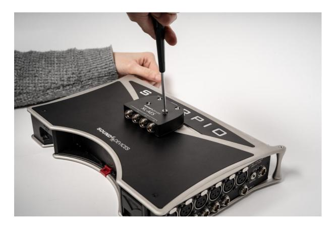
Attach the connector cover to the bottom for safekeeping.
