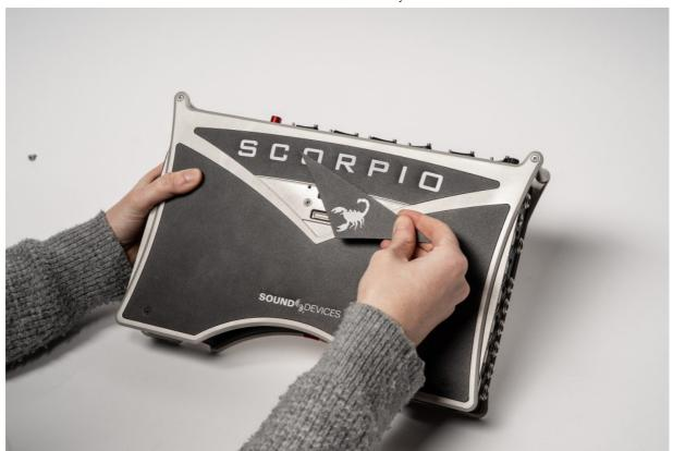
If you are installing the XL-AES on a Scorpio, peel and stick the included gasket to the bottom of the XL-AES before mating with the Scorpio.
