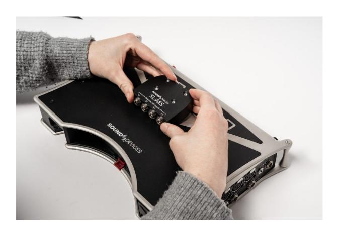
Using the included screws, attach the XL-AES to the host mixer-recorder. On the 833 and 888, the longer 25mm screws go in the front two holes. On Scorpio, the longer screws go in the back. Use the two remaining 8mm screws to cover the unused holes in the XL-AES.
