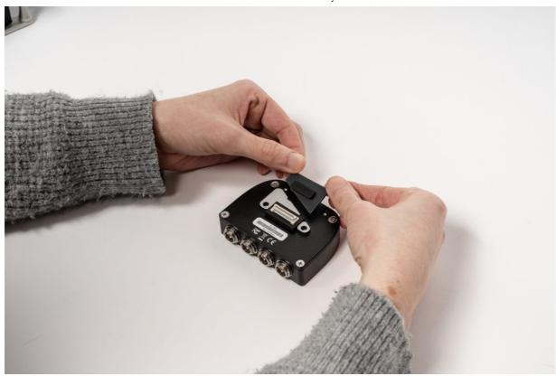
Align the connector on the bottom of the unit with the proper connector on the top panel of the host mixer/recorder.
