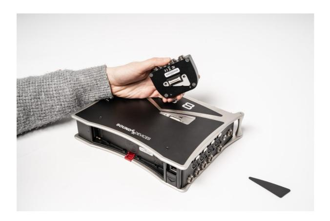
Carefully push the XL-AES onto the host mixer with care and attention to the alignment of the connectors. There will be no gap between the XL-AES and the host mixer/recorder when installed properly.
