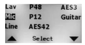
The A20-TX is compatible with many types of input sources.
