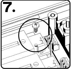
Remove the top screw of the fader
