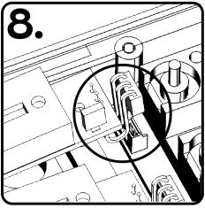
Disconnect the fader connector
