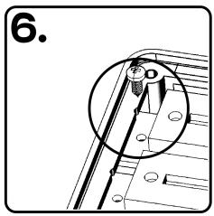
Remove the bottom screw of the fader
