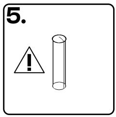
Keep the light guides apart At reassembly, put these back after installing the front panel
