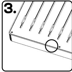
If necessary, use a tool such as a flat screwdriver to lift the front panel from the designated location
